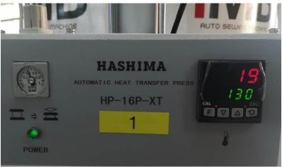
Press, Turn on the ironing machine, the green number is the set temperature, and the red number is the real-time temperature,
