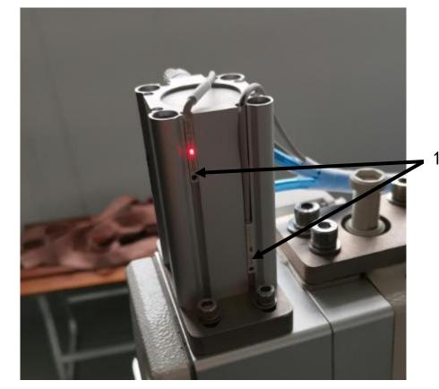
6.3 Position adjustment of cylinder magnetic switch
