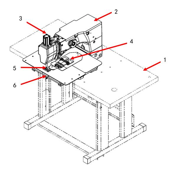
1: Table stand;2: Machine head;3: Upper die assembly;4: Feeding assembly;5: Lower die assembly;6: Dust collecting module;
