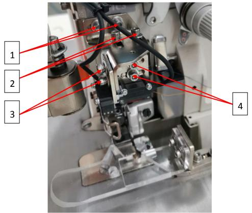
As shown above: Screw 1 adjusts the front and back positions of the sensor of the opening seam and the rotary drop hammer at the same time;
