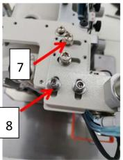
As shown above, Screw 7 adjust the left and right position of the drop hammer point; Screw 8 adjust the front and rear position of the drop hammer point;
