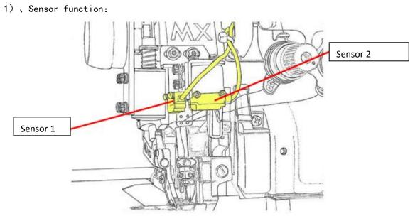
Sensor 1: Start sewing when fabric is detected. Sensor 2: Drop the hammer when the cloth is not detected. In this way, the circular arc sewing of cloth can be realized. When the signal is not detected by the No.1 optical eye, the sewing stops after the cutter cuts the thread.
