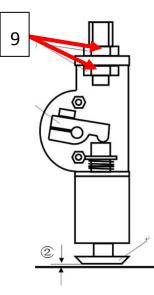
As shown above, Adjust the lowest position of the falling hammer device after the falling of the screw 9, so that the gap between the falling hammer and the platform plate 2 is slightly smaller than the thickness of the sewn cloth;
