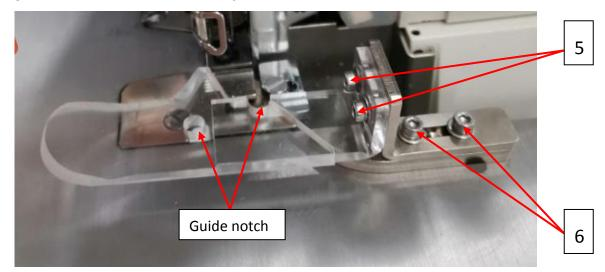
As shown above: Screw 5 adjusts the up and down position of the guide plate to make the cloth flat and smooth;
