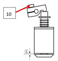
As shown above, Screw 10 adjusts the position of the falling hammer device after lifting, so that there is a certain gap between the falling hammer and the fixed block after lifting, 1 to avoid collision and impact noise, and the gap is about 1mm, which is the best;
